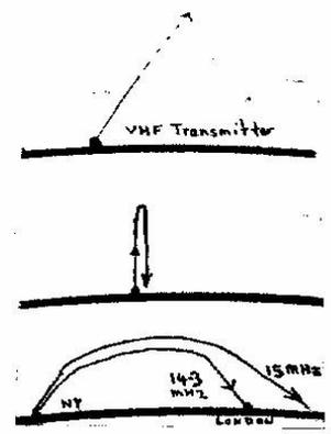
**The Critical Frequency** is the highest frequency signal that, when transmitted straight up, will be *reflected* (total refraction) back to earth at the same point.
