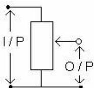
I am sure that you use a potentiometer many times each day..... Think of the volume control on your radio. The sound will be loudest when the wiper is at the top and quietest when it's at the bottom. By convention, the pots are wired so that turning clockwise, moving up or to the right will increase the output.
