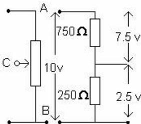
As an example 10 volts is connected across a 1000 Ohm potentiometer. ( A & B ) The voltage between B & C will be proportional to the position of the wiper. If it is one quarter round the track, starting from the bottom, then potential difference between B & C will be  $10 \times 1/4 = 2.5 \text{ V}$ . An equivalent potential divider could be made with two fixed resistors.
