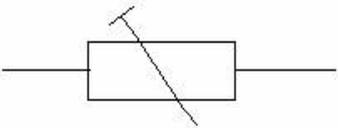
This symbol represents a variable resistor that it mounted within the equipment, Usually on the printed circuit board. It is adjusted by a screwdriver when the equipment is being aligned or maintained.
