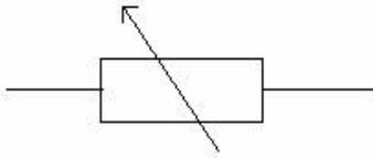
This symbol represents a variable resistor that is adjusted by a knob on the front panel. I.E. This component is adjusted during the normal operation of the equipment
