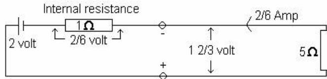
For Example, a 2 volt lead acid cell is connected across a 5 Ohm resistor. The cell has an internal resistance of one Ohm.
