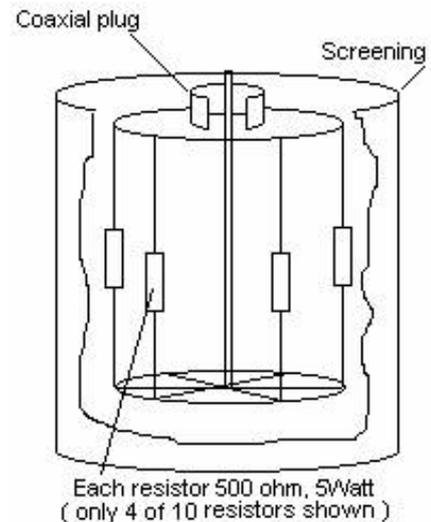
The 50 Ohm dummy load shown here, Has ten resistors connected in parallel. Each resistor is 500 Ohm and is rated at 5 Watts. It would Handle 50 Watts continuously and 500 Watts for short periods.
