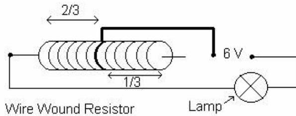
If the total resistance of the carbon track is 30 K $\Omega$  then the resistance between the wiper and the top connection would be 10 k $\Omega$ . If The wiper is moved to the top and then the bottom the resistance would be 0 Ohms ( Short circuit ) and 30 K $\Omega$  respectively.
