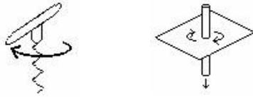
Maxwell's right hand corkscrew rule gives the direction of this field: If a right hand corkscrew moves forward in the direction of the current then its rotation will indicate the direction of the magnetic field.
