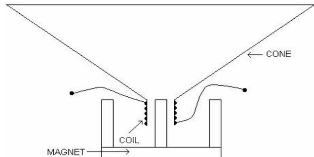
The movement of the diaphragm (or the cone) vibrates the adjacent air. We hear these vibrations and call it sound.
