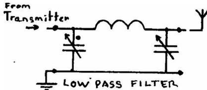
The network is connected between the aerial socket of the transmitter and the aerial wire. It is very effective in reducing harmonics. It is four times better than a simple parallel tuned circuit for reducing the second harmonic and nine times better at the third harmonic.
