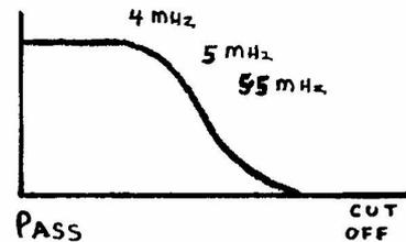
This filter could be used in an 80 Metre (3.5 -3.8 MHz) transmitter.
