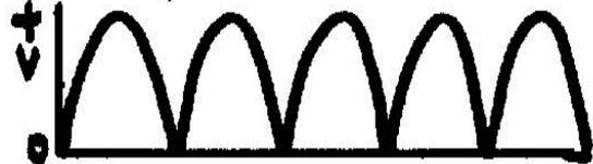
(For a negative output all the diodes would be reversed.)
